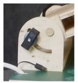
To compare these two latitudes, you will collect data on the same day. First, set the angle on the small base protractor. The small base protractor reflects both latitude and time of year.
