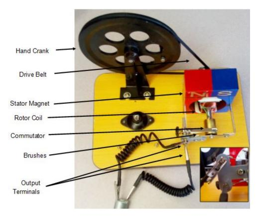
Without the motor or lamp connected, turn the hand-crank generator.
