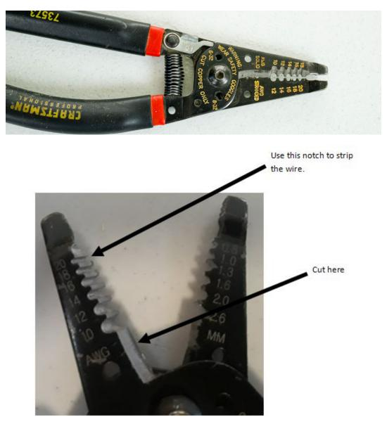
Measure the right length of wire by holding it between the two connections. A bit too long is better than a bit too short.
