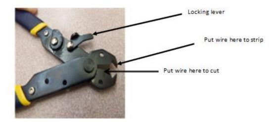
Adjust the cutter to strip the wire by turning the little dial on the side. It should be set on 20. This dial keeps the jaws open just enough so the V-shaped part will cut through the plastic coating but not through the wire itself. You can use a small piece of tape to help keep the dial set.
