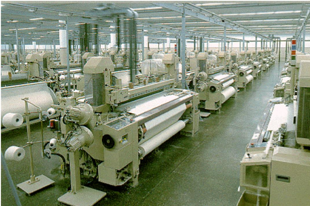
An electric loom uses a centralized motor, so any belts or shafts can be contained within the machine to keep workers safer.
