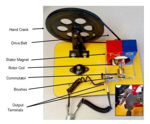
Turn the crank on the generator. What part spins most and what parts do not move at all?
